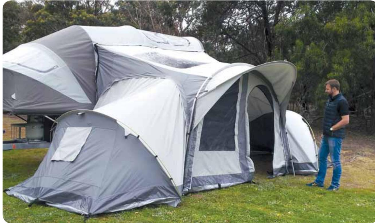
Engineered for all-terrain travel and providing comfortable accommodation under any conditions, the Opus' tent is modular in design in so far that an additional awning can be joined to the main tent, creating an extension that measures a full 2m wide. For even more room, a pair of inner extension pods can be attached, gaining you another 2.4 of covered living space, so there's plenty of room for family and friends keen to tag along on your next bush adventure.
