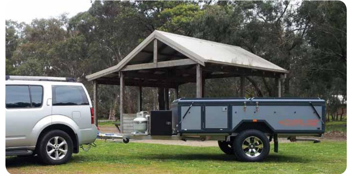
Your chassis on the Opus is hot-dip galvanised to effectively seal it with a super-tough coating designed to resist corrosion and rust. The extended drawbar is made from 100mm x 50mm sections of steel and is fitted with dedicated holders for two jerry cans, a lockable holder for carrying one 9kg gas bottle and a front-mounted toolbox perfect for packing along extra camp gear.
