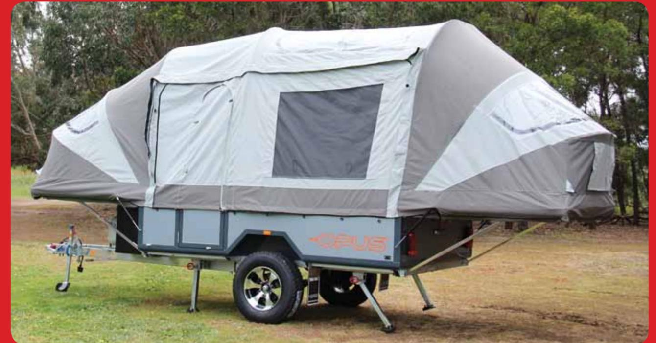
The tent on the Opus is made from a heavy-duty, 400gsm micro-weave poly/cotton blend canvas that combines the high breathability and water-tightness of cotton with the strength and water resistance of polyester. When erect, the tent helps to create the Opus's high ceiling effect that gives you heaps of functional living space inside.
