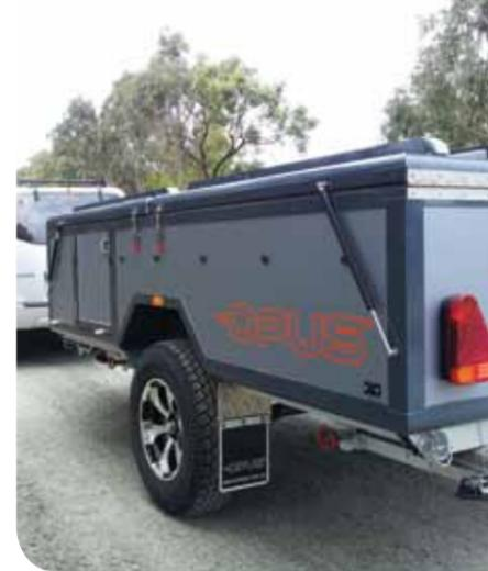
With the inclusion of a rugged, five-leaf off-road suspension and electric disc brakes, with off-road magnets. The Opus has been engineered from the bottom up for true blue Aussie action and adventure. The Opus cruises on 15in, five-stud alloy wheels and all-terrain tyres so it can be trusted to perform even over tough tracks and heavily corrugated roads.
